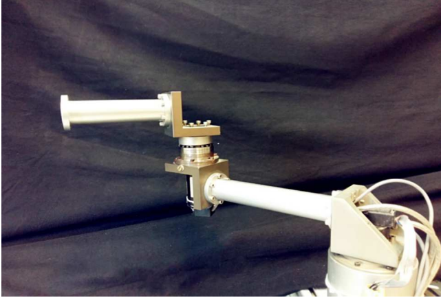
Fig. 1: The 2-DoF Robot Manipulator for the Experiment
