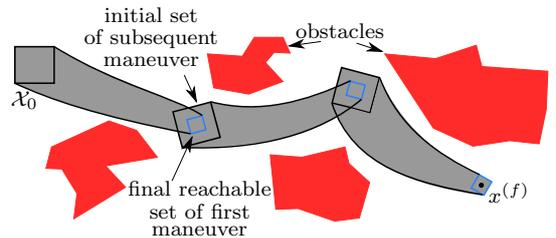
Fig. 1. Using maneuvers (gray) to steer all states from  $\mathcal{X}_0$  to  $x^{(f)}$  while avoiding nonconvex obstacles (red). The final set (blue box) of one maneuver is always contained inside the initial set (black box) of the following maneuver.
