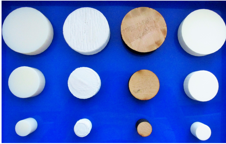
Figure 5.4: Three different-sized cylinders out of four different materials from left to right: photopolymer, ABS, wood and PA.
