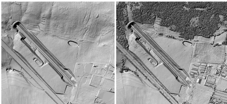
Fig. 1. Left: DTM, Right DSM. Data obtained from airborne laser scanning, resolution 1 m, area covers 1000x1000 m and shows a part of Germany's high-speed train network between Nuremberg and Ingolstadt. Image courtesy Wolfgang Reinhardt and Walter Henninger (Munich).
