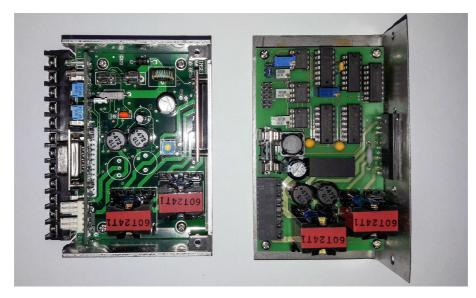
Figure 2.6: Photograph of the original (left) and modified (right) motor driver.
