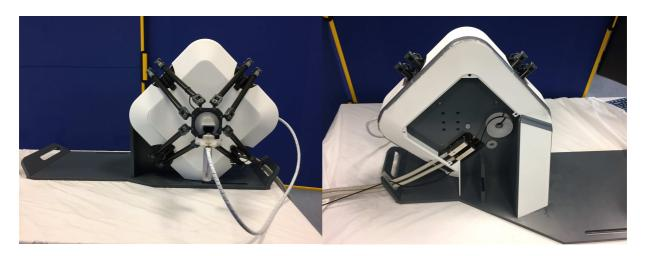
Figure 4.10: Photographs of the MR-Octo from front (left) and back (right). The backside can be closed entirely by the chassis, which is not depicted.
