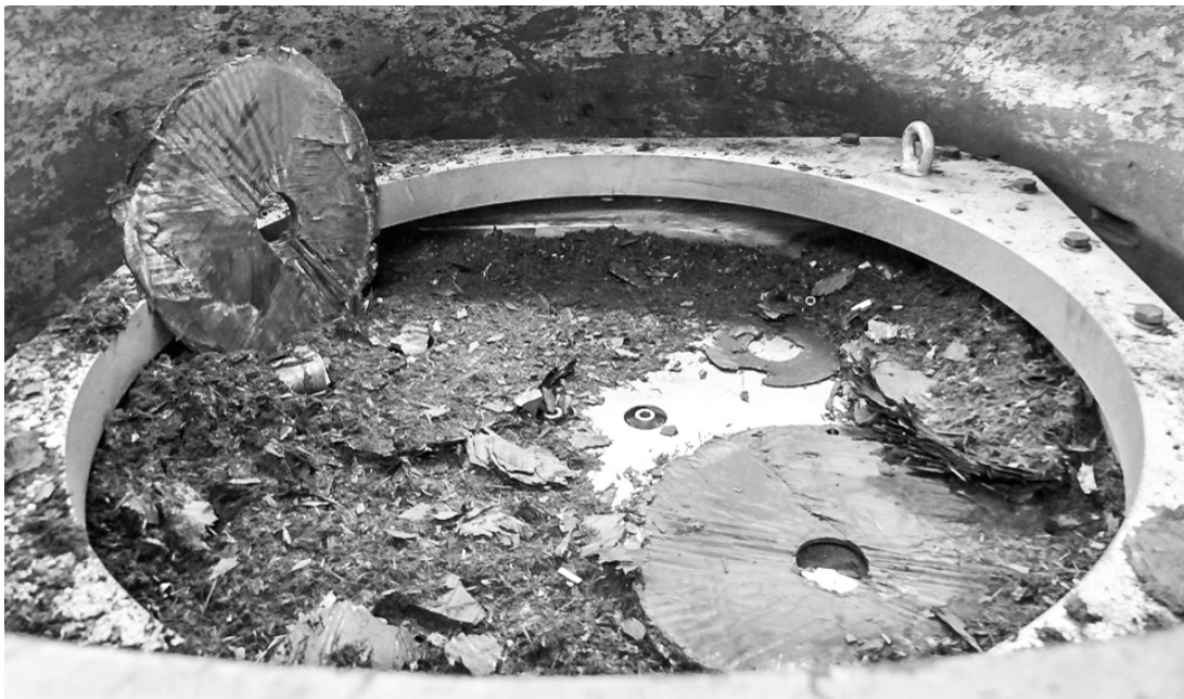
Figure 7.15.: Destroyed chopper disk after spinning strength test at overspeed [145].
