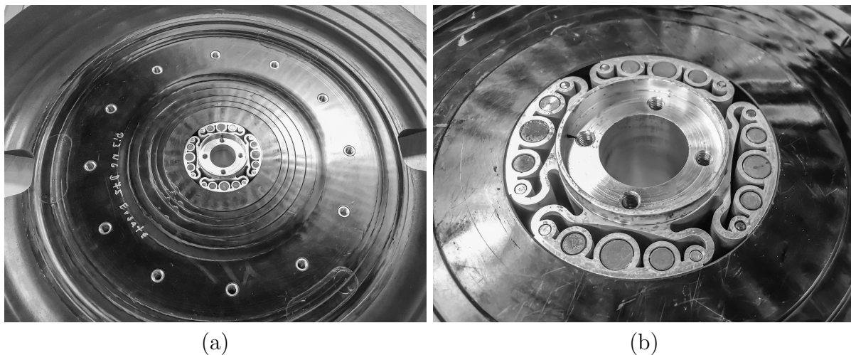
Figure 7.13.: Application of the new hub in a CFRP disk, (a) overview of the assembly, (b) detailed view on the hub with tungsten weights.
