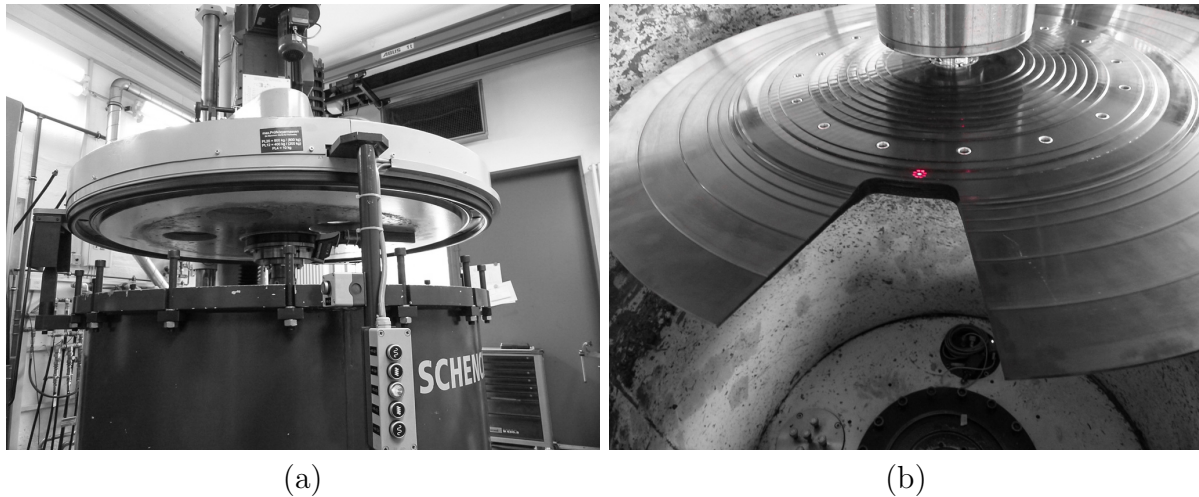
Figure 7.9.: Overspeed test stand BI 4 by Schenck, (a) test stand with mounted CFRP disk, (b) applied pyrometer for a non-contact temperature measurement during rotation.
