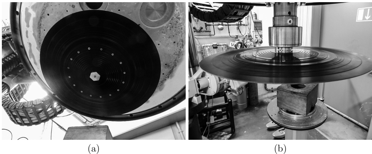
Figure 7.10.: CFRP disk without cut-outs, (a) view from the bottom and (b) disk mounted on the shaft and assembled in the spinning test machine.
