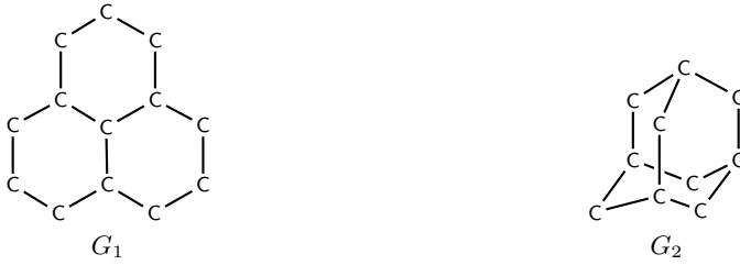
Fig. 3. Molecules \mathbf{G}_1 (Perhydrophenalene) C_{13}H_{22} and \mathbf{G}_2 (Adamantane) C_{13}H_{16} . All edge weights are assumed to be equal to one. The minimum cycle basis of \mathbf{G}_1 consists of the three hexagons. Since they are unique, each hexagon represents its own \sim_6 equivalence class. In \mathbf{G}_2 , any three of the four visible hexagons add up to the fourth, hence they are all interchangeable. Any three of them form a minimum cycle basis.
