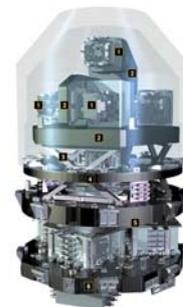
Figure 4. Drawing of the GOCE gradiometer
