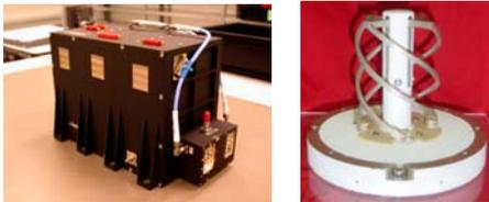
Figure 5. The GOCE GPS receiver and antenna (SSTI)
