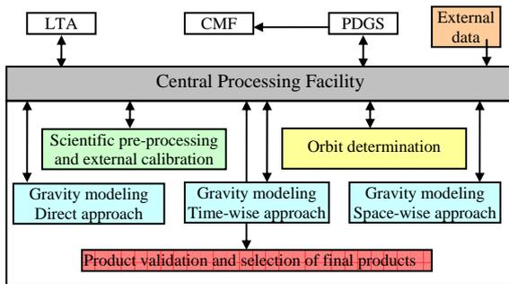
Figure 3. High-level architecture of the HPF. The CPF is the central node for all data flow along the internal and external interfaces.
