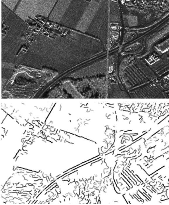
Figure 7 Assessment of a line extraction (below) from a sub-urban SAR scene (above)
