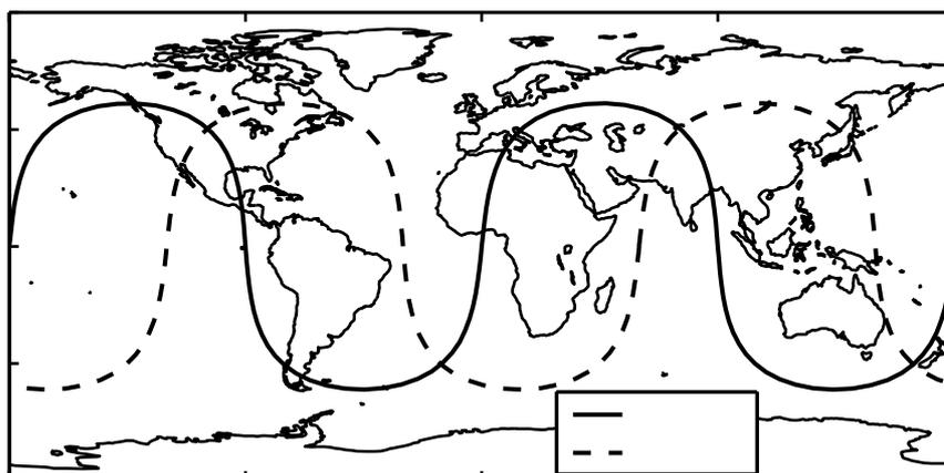
Figure 5.6: Ground tracks of two GPS satellites
