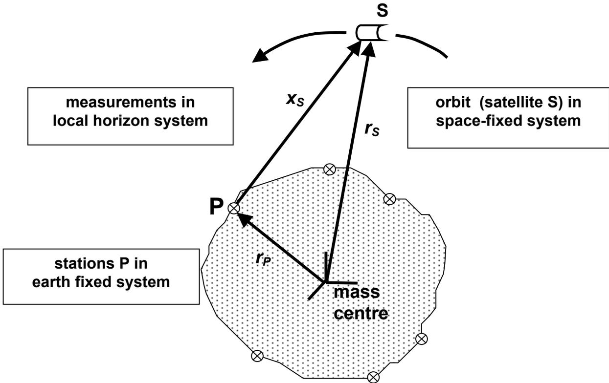
Figure 3.1: Vector sum of geocentric point position vector, topocentric measurement vector and geocentric satellite orbit vector, each one expressed in a different reference system.
