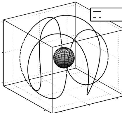
Figure 5.4: The orbits of two satellites in an earth-fixed geocentric coordinate system
