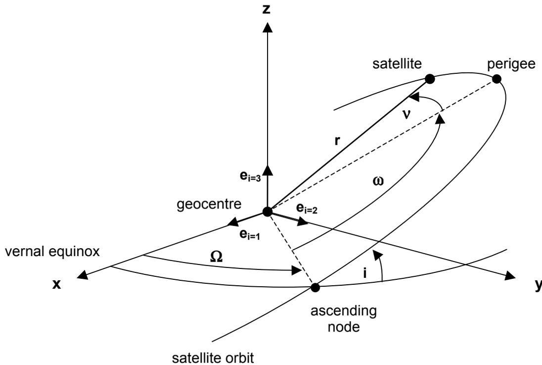
Figure 5.2: Orbital orientation in a space-fixed coordinate system
