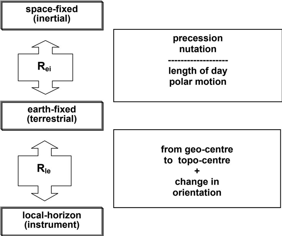
Figure 2.1: Hierarchy of reference systems - from space-fixed via earth-fixed to local horizontal
