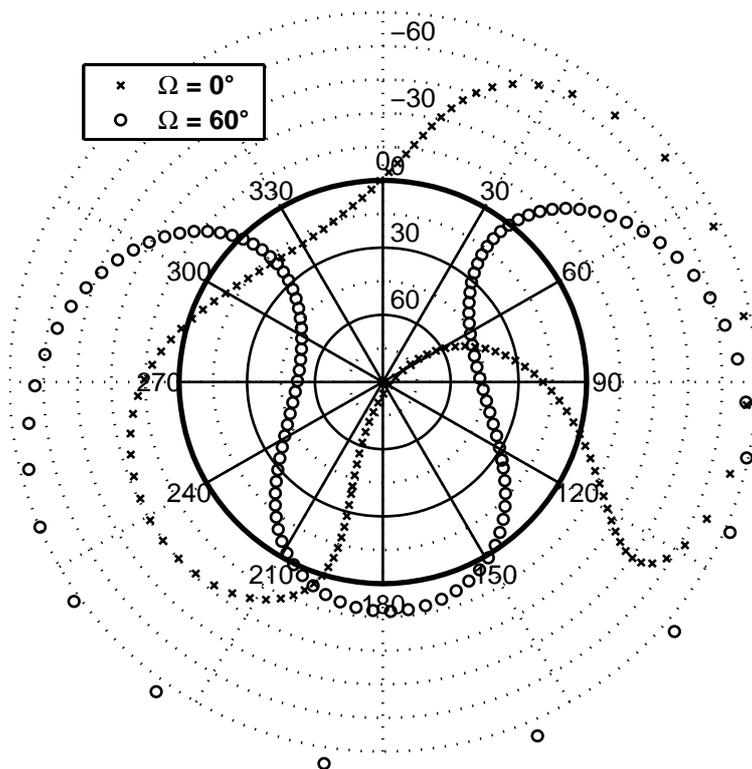
Figure 5.5: Sky plot or visibility plot, centered at Alpbach ( $\varphi = 47^{\circ}24'N$ ,  $\lambda = 11^{\circ}57'E$ ), with traces of two GPS satellites
