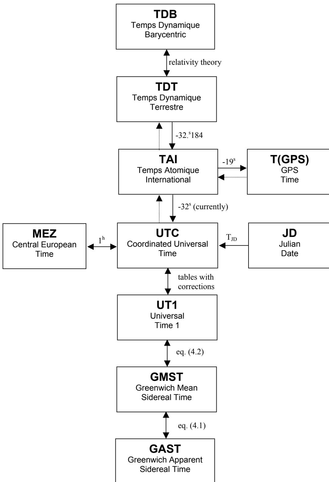
Figure 4.1: Transformation between time systems (after: MÜLLER, 1999)
