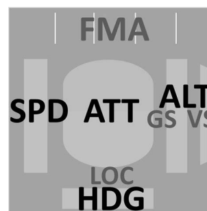
Fig. 2 Areas of interest on the primary flight display considered in this study ( black letters ): speed ( SPD ), attitude ( ATT ), altitude ( ALT ) including the glideslope indicator ( GS ) and vertical speed ( VS ), and heading ( HDG ) including the localizer indicator ( LOC ). Some areas ( GS , VS , LOC ) could not be separately considered due to eye-tracking accuracy. The flight mode annunciator ( FMA ) was not considered because no automation modes were used
