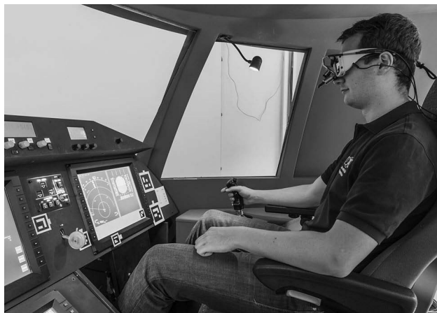
Fig. 1 Simulator setting showing a participant with mounted shutter glasses and eye tracker
