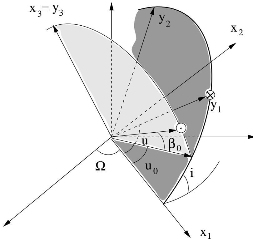
**Figure 3.** Positions of satellite and sun.  $u$  and  $u_0$  are the arguments of latitude of satellite and sun,  $\beta_0$  is the elevation of the sun above the orbital plane;  $\Omega$  is the right ascension of the ascending node of the satellite's orbital plane.
