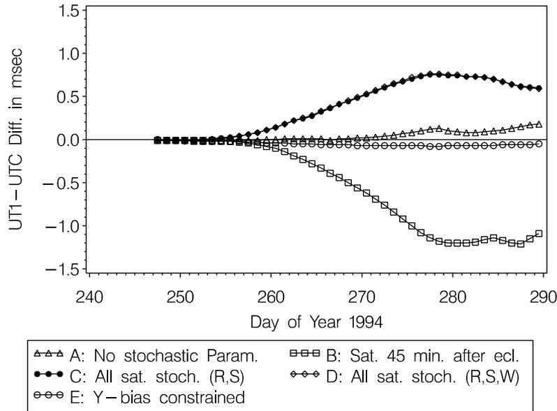
**Figure 5.** Mean rotation of the nodes computed from the  $y$ -bias parameters estimated using different orbit strategies
