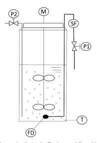
**Figure 1.** Propagation device for *Torulaspora delbrueckii* propagation. M = motor for agitator; P1 = time controlled aeration pump; P2 = sampling pump; T = temperature transmitter; FD = filter disc; and SF = sterile air filter.
