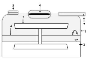
**Fig. 1.** Schematic diagram of the Speedy Breedy minifermenter (1): YM broth (2), magnetic stirrer (3), stirrer axis (4), inoculation rubber septum (5), measure membrane (6), and pressure-measuring connection to the Speedy Breedy device (7).
