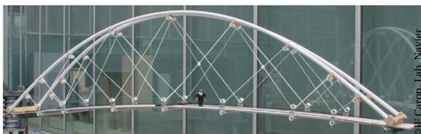
**Figure 4.7:** Mock-up of the selfstressed bowstring footbridge in scale 1 : 10 (©J.-F. Caron [40], used with kind permission)
