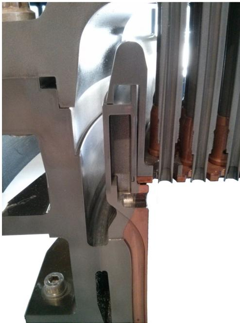
(a) L-shaped quarter-wave resonator in a Vulcain 2 engine.<sup>1</sup>
