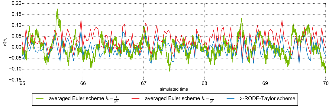
Figure 12.7.: Comparison of expected values E(\tilde{u}) using 2^{10} path-wise solutions for the KT model over the arbitrary time interval [65, 70] obtained by three different solver scenarios: The green and red expected values stem from solutions obtained by the averaged Euler method with h = \frac{1}{2^{10}} and h = \frac{1}{2^5} , respectively. The blue lines corresponds to solutions from the 3-RODE-Taylor scheme h = \frac{1}{2^5} . \delta = \frac{1}{2^{20}} for all three RODE solutions.
