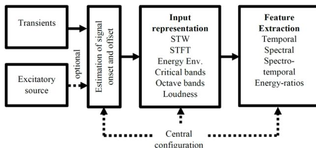
**Figure 2:** Stepwise process from input to features as done by FETT. Input from excitatory source (e.g. impulse hammer) is optional. A central configuration table stores all necessary parameters for estimation of signal boundaries (onset and end), input representation and feature extraction.
