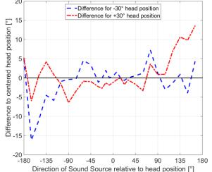
**Figure 2:** Differences of median localization results for non-centered head orientations (blue, dashed line:  $-30^{\circ}$ ; red, dash-dotted line:  $+30^{\circ}$ ) to  $0^{\circ}$  head-above-torso orientation.
