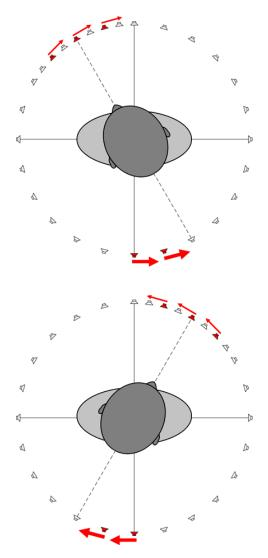
**Figure 3:** Observed localization shifts, indicated by arrows, for exemplary sound directions, marked in red. The upper drawing visualizes observed shifts for  $-30^{\circ}$  head orientation and the lower drawing for  $+30^{\circ}$  head orientation. The black dotted line indicates the median axis.
