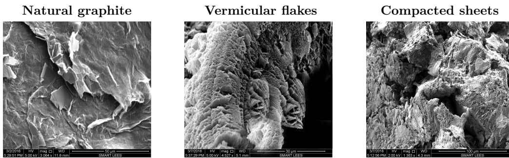
Figure 5.11: Steps of expanded graphite production
