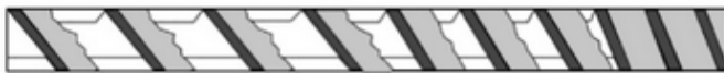
Figure 16: Effect of conveying elements with different pitch on filling degree in free screw volume. Reprinted from Giles et al. (2004) with permission of Elsevier.
