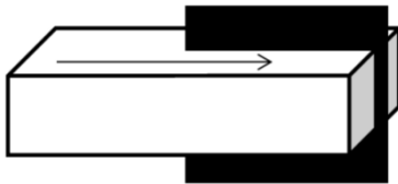
Figure 42: Sample preparation for assessing the anisotropic structures. The black rectangle indicates the cutting side used for assessing the flow profile. The arrow indicates the flow direction of the extrudate.
