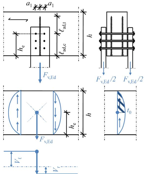
Figure 7: Reinforced cross-connection: reinforcement (above) and distribution of shear stresses and shear flow (below)
