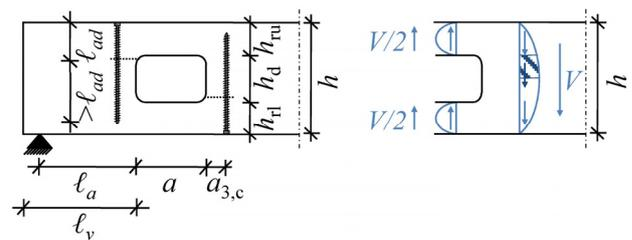
**Figure 6:** Hole in beam: reinforcement (left) and distribution of shear stresses (right)
