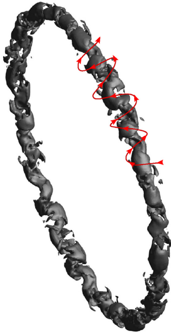
Fig. 7. Vortex ring with Widnall-type instability in the long-term evolution of ISBI ( Ma = 2.83 ) at t = 600 \mu\text{s} .
