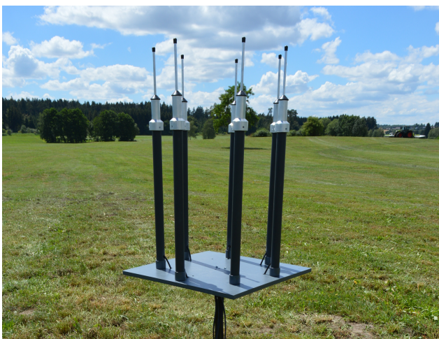
Figure 8. Picture of the measurement setup in an open wide and flat meadow area for far-field measurements.
