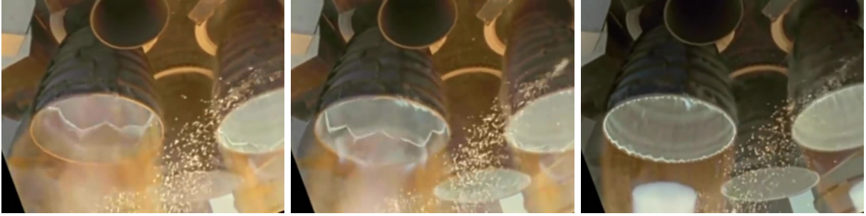
Figure 1.1.: Transient start-up of the SSME. Courtesy of NASA.
