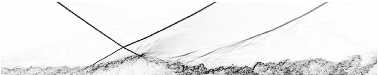
Figure 1.3.: Numerical schlieren image from a LES showing contours of the density gradient magnitude |\nabla\rho| for an impinging SWBLI at Ma = 3 and Re_\delta \approx 2 \cdot 10^5 .
