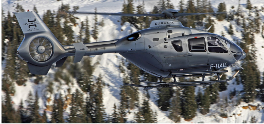
Figure 1.2: Airbus Helicopters H135 equipped with a Fenestron tail rotor [3].
