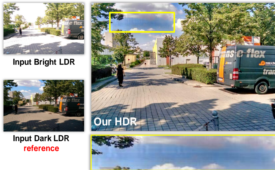
Figure 5.25: Example of the resulting HDR image using our Double-Loss FC-FlowNet -inspired HDR rendering model. In this case, the region depicting the sky details contains some artifacts. This might be explained by the fact that the initial training as well as the free-motion-set do not cover such cases sufficiently. However, the dynamic range of the remaining parts of the scene is successfully enhanced, which in turn improves the overall visual quality as shown in the output HDR image.
