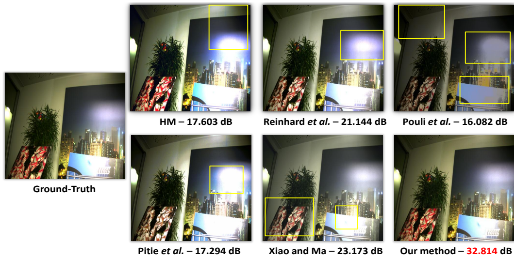
Figure 4.7: Zoom-ins on color mapping results from various methods including our approach. The results correspond to the 5 th testing sequence from the uEye dataset. The yellow boxes indicate areas of faulty color mapping results.
