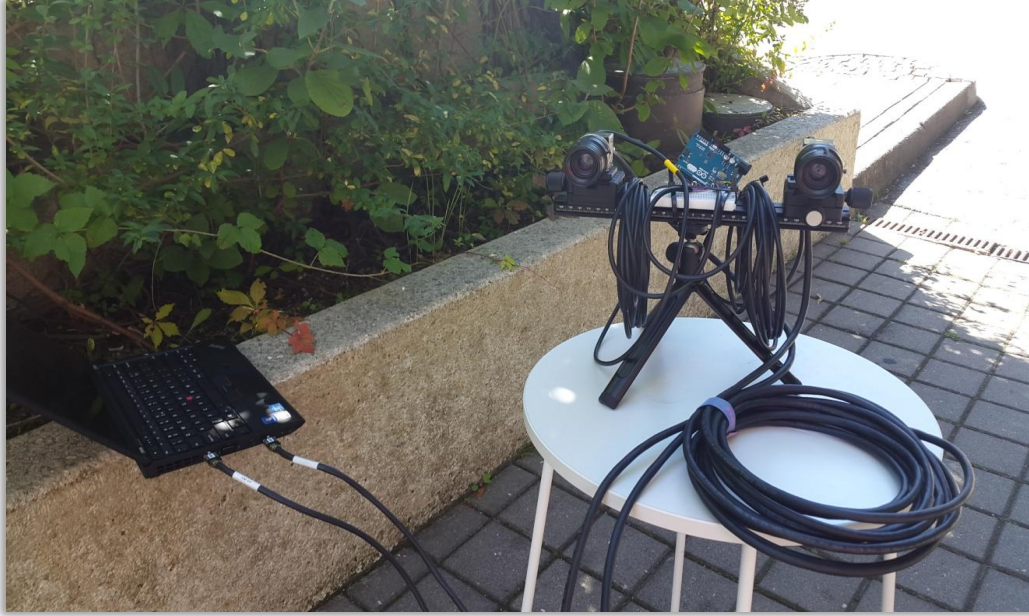
Figure 5.4: Stereo setup composed of 2 IDS uEye cameras used for the purpose of creating the outdoor dataset.
