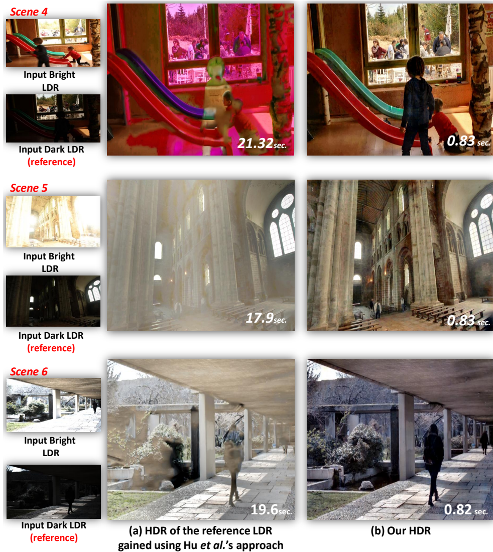
Figure 5.24: Visual Comparison between the rendered HDR images using the method of Hu et al. [15] (column a ) and our HDR from the final third experiment (column b ). In addition, we provide the corresponding execution times of both approaches. Note that the computation time of Hu et al. 's approach apply only to the alignment part. Once again, our HDR rendering model learned on the full stack of available HDR images is capable of successfully processing extreme cases where large motion occurs in the saturated areas. Input images of scene 4 are courtesy of [7] and images of scenes 5 and 6 are courtesy of [3].
