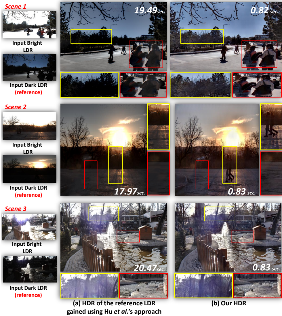
Figure 5.23: Visual Comparison between the rendered HDR images using the method of Hu et al. [15] (column a ) and our HDR from the final third experiment (column b ). In addition, we provide the corresponding execution times of both approaches. Note that the computation time of Hu et al. 's approach apply only to the alignment part. Despite the large difference in terms of scene content as well as exposure ration between the input LDR, our HDR model is able to effectively extend the dynamic range of the reference image while restraining all kinds of artifacts related to HDR rendering on dynamic scenes. This is more noticeable on the zoomed-in areas. Input images are courtesy of [3].
