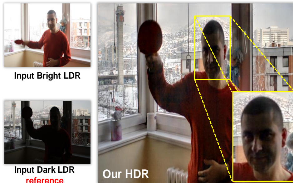
Figure 5.26: Example of the resulting HDR image using our Double-Loss FC-FlowNet -inspired HDR rendering model. As shown in the highlighted area, the details corresponding to the face region were not fully recovered from the non-reference image. This implies that the transfer of texture in this example was not efficient. However, the dynamic range of the remaining parts of the scene is successfully enhanced, despite the fast motion inherent to the scene. Input images courtesy of [7].
