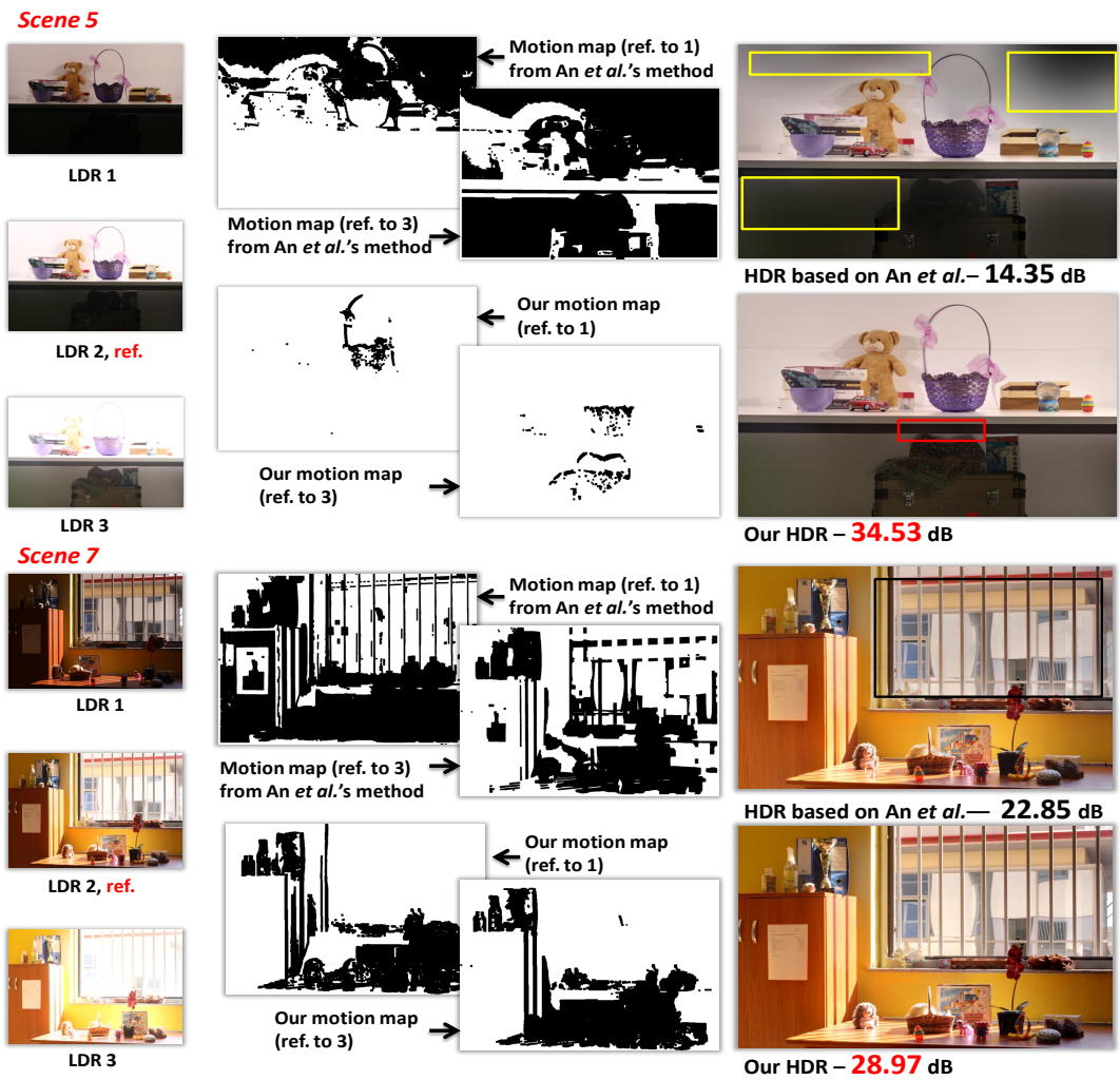
Figure 2.11: Comparison of the results generated using the approach described in [5] together with our results. The accurate and relatively noise-free binary motion maps computed using our method significantly improve the visual quality of the final HDR. This explains the large difference between both approaches in terms of PSNR values. Areas under the yellow boxes represent regions where the inaccurate motion detection from [5] negatively impacts the final HDR. Red boxes indicate regions where our algorithm creates artifacts. Input images are courtesy of [1].
