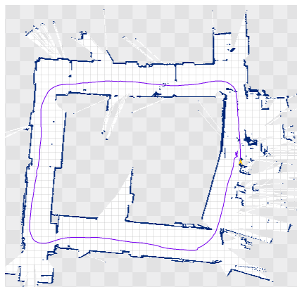
Fig. 1.5: The inability of the algorithm in detecting the loop closure constraint in context of laser based SLAM leads to an inconsistent metric map of the environment.
