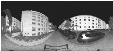
(j) Equirectangular intensity image of point cloud acquired during night time at the same location as in Figure 4.21(g)
