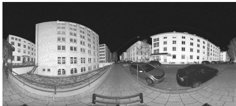
(g) Equirectangular intensity image of point cloud acquired during day time
