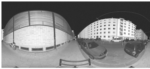
(a) Equirectangular intensity image of a point cloud acquired during night time
