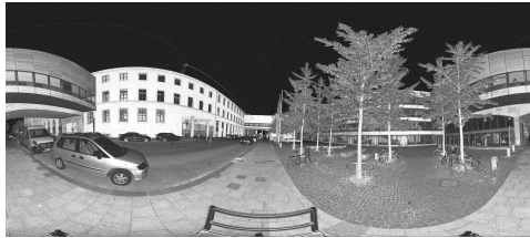
(d) Equirectangular intensity image of point cloud acquired during night time at the same location as in Figure 4.21(a)
