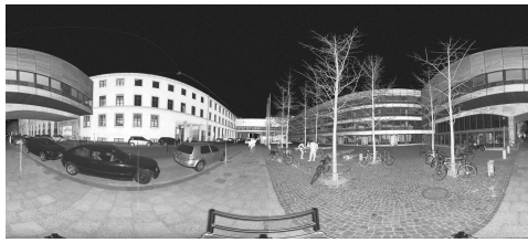
(a) Equirectangular intensity image of point cloud acquired during day time
