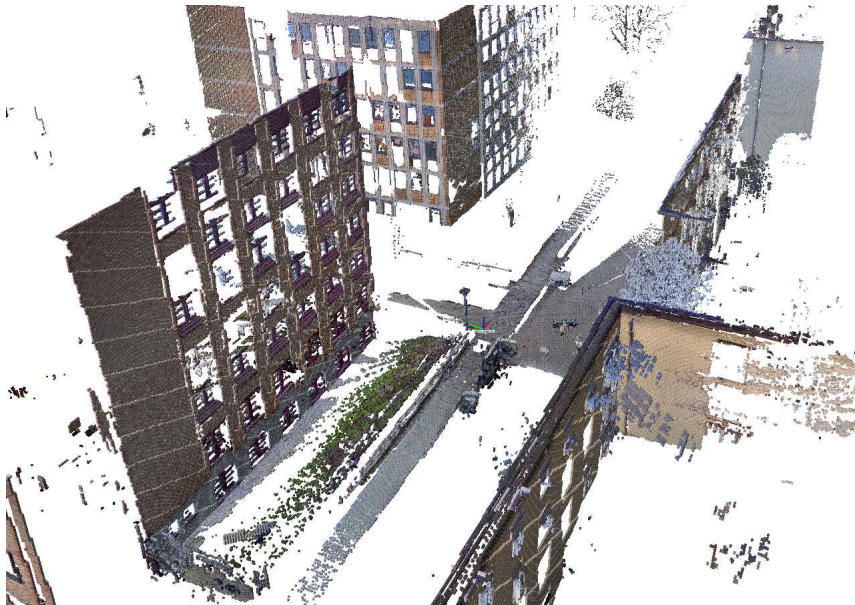
(c) Grid based representation (10 cm grid cell size) using the Rtree occupancy grid [89, 211] with color information
