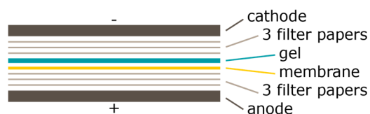
Figure II-2: Assembly of Western blot stacks for semi-dry blot.
