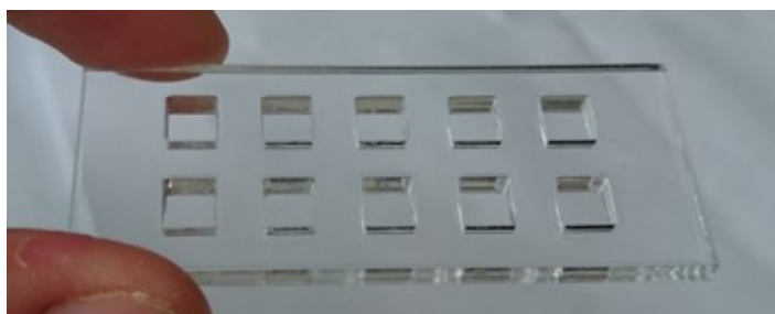
Figure 3.6: Acryl-glass mold for 3D hybrid-gel molding.
