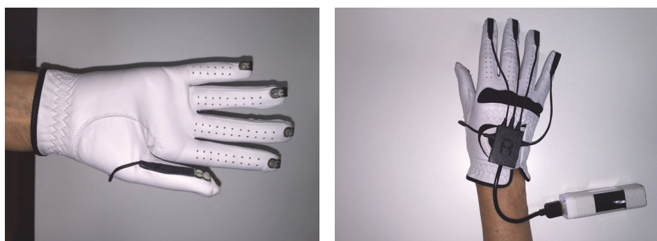
FIGURE 3: Teacher's glove with integrated pressure sensors.
