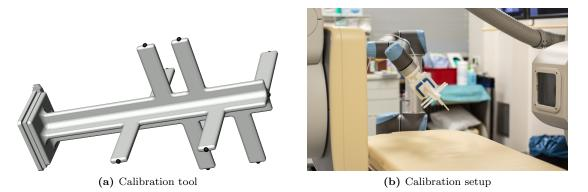
Figure 9.2: a) CAD drawing of the calibration tool and b) setup used to map the C-arm coordinate system to the robot coordinate system. The spheres attached to the fins appear prominently in the CT volume and can be easily segmented[90].
