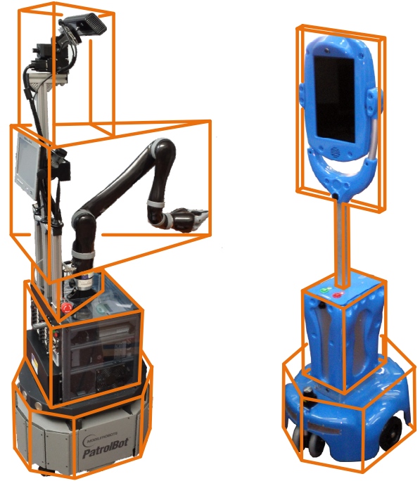
Figure 5. Example of 3D geometric models of the Giraff robot (right) and Rhodon (left)
