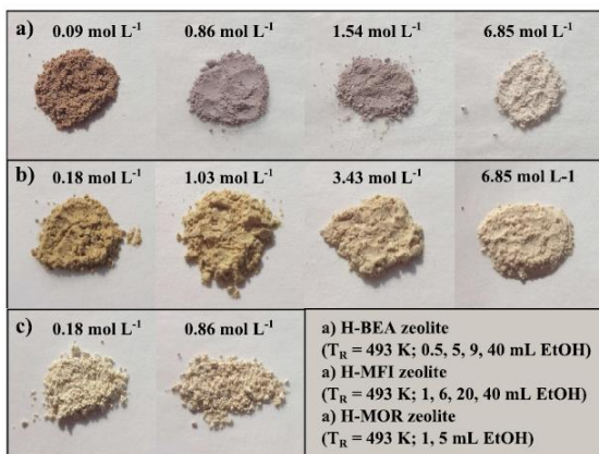
Figure 4.14: Images of spent catalyst. a) H-BEA, b) H-MFI and c) H-MOR
