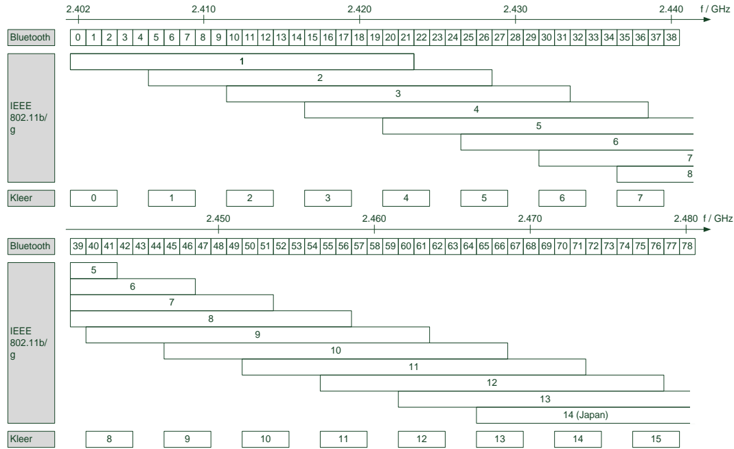
Figure 2. Bluetooth, IEEE 802.11b/g and KLEER channels in the 2.4 GHz-ISM-band.
