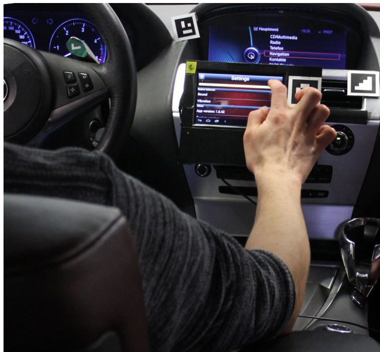
Figure 4.2.: Laboratory setup for the evaluation experiment. Touchscreen tablet (in use). The on-board screen for rotary knob interactions is above. The rotary knob is visible in the lower right corner
