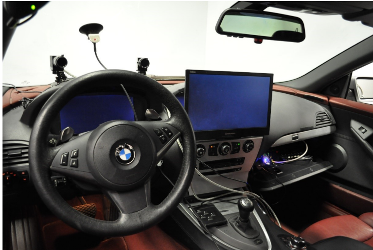
Figure 4.2. – Experimental setup inside vehicle mock-up. The monitor placed in the console was used to display the SuRT. SuRT manual inputs were communicated through the numeric keypad located to the left of the gear shift. Near the windshield, 2 cameras (not relevant for this experiment) and an LED (used for EEG calibration) can be seen attached to the windshield via suction cup. The suction cup was removed after the calibration was performed prior to experimentation.
