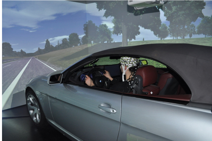
Figure 4.1. – Experimental setup; participant with EEG cap and active electrodes inside the vehicle mock-up.
