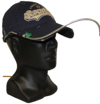
(a) Head-mounted DRT (HDRT)
