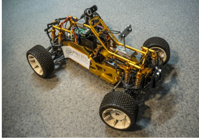
Figure 5.1: The overview of the model car. Its size is 120\text{ cm} \times 70\text{ cm} \times 35\text{ cm} and its weight is around 20 kg
