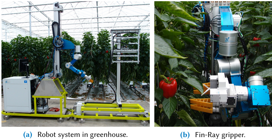
Figure 2.5: Final prototype of the CROPS sweet pepper harvesting robot system in a greenhouse at Wageningen, Netherlands (Hemming, Bac, Tuijl, et al. 2014).
