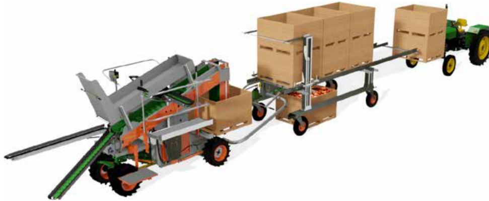
Figure 2.1: MUNCKHOF PLUK-O-TRAK harvesting aid pulled by a tractor through the orchard. Human pickers place the fruit on the conveyor belt system on the left, which automatically transports them into a storage container. Image taken from Munckhof (2016).
