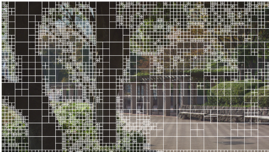
(c) CU structure of the original encoding
