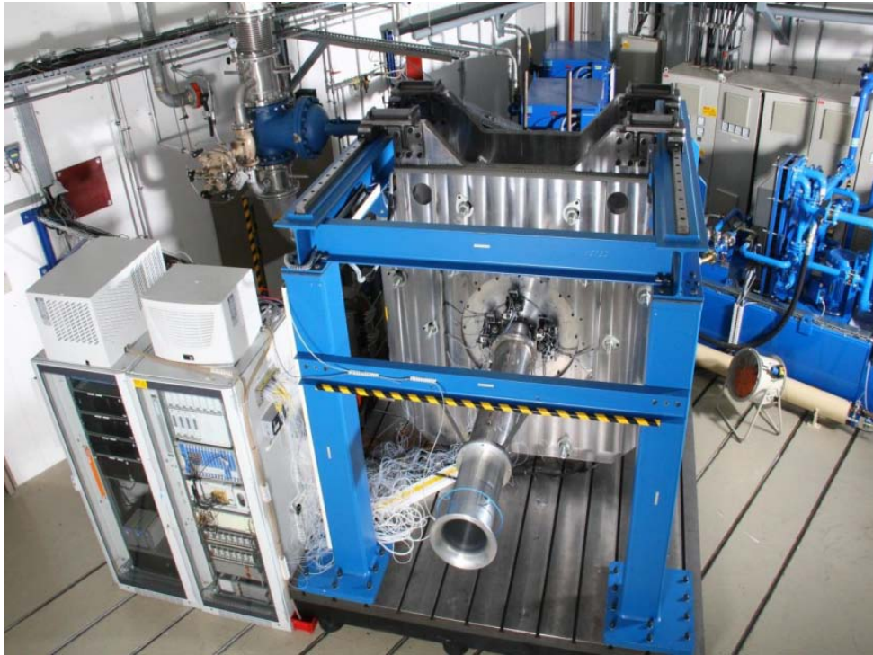
Figure 3.1: TUM-LFA centrifugal compressor test facility from Lang [59]
