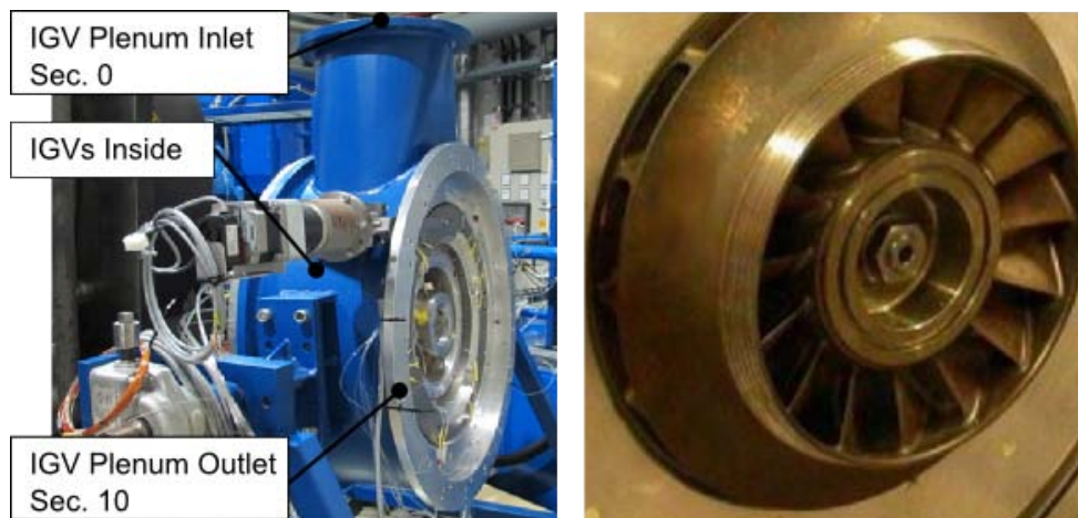
Figure 3.4: IG V plenum for the rotating test (left) and the impeller (right) from Guidotti [43]
