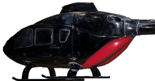
Figure 6.37: Contoured strakes as cast silicon parts (red) mounted on F1M0L1.
