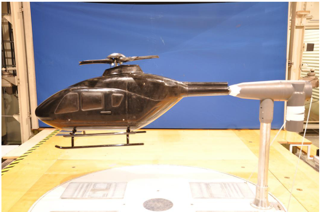
Figure 2.8: Complete baseline model installed on the tailboom model support in the test section of WTA.
