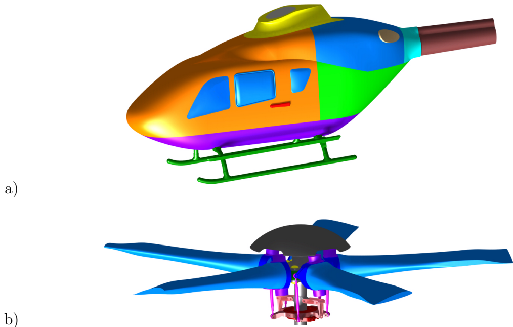
Figure 2.2: Segmentation of the ADHeRo wind tunnel model in its baseline configuration. a) Fuselage and skid-landing-gear, b) rotor head. (For a improved visualisation, the scale of figure b) is increased compared against figure a).
