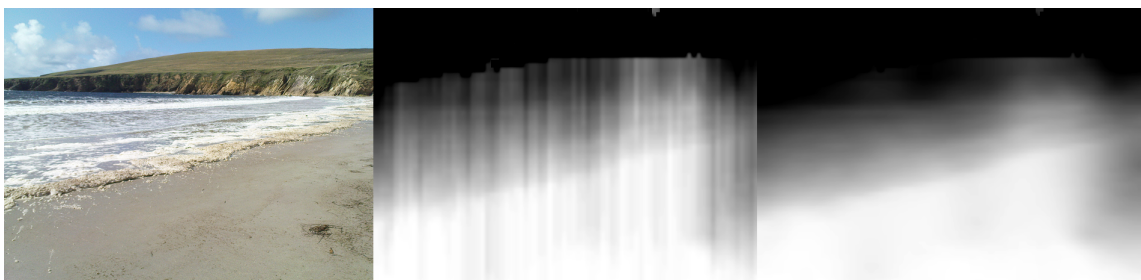
Figure 5.3.: Texture based depth map of a beach scene. There are visible vertical stripes caused by error propagation. Sky removed by the sky detector. Left to right: original, unfiltered, filtered.
