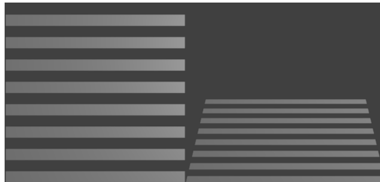
Figure 5.2.: The same surface pattern viewed from two different angles. Features are closer to each other when viewed from a steeper angle.
