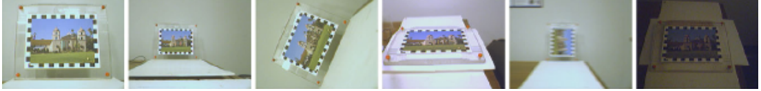
Figure 6.6.: Some example frames displaying the different motion patterns. From left to right: the first two images show a scale change, rotation, perspective distortion, motion blur and lightning. The evaluation uses only the area inside the black-and-white border pattern.
