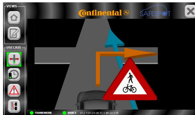
Figure 7.44 Continental HMI for the scenario pedestrian or bicyclist on the right side [PU ET AL., 2010]
