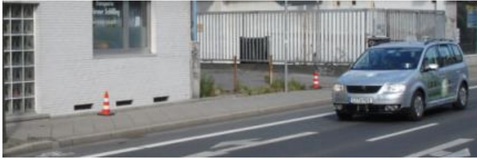
Figure 7.50 Traffic cones at the roadside for marking the distance during the tests
