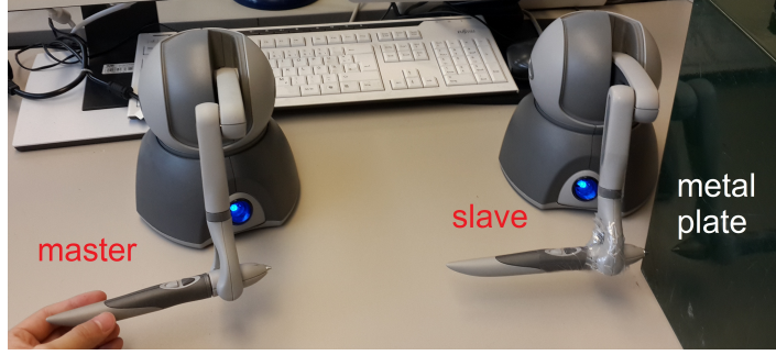
Figure 3.5: Teleoperation setup with adjustable time delay.
