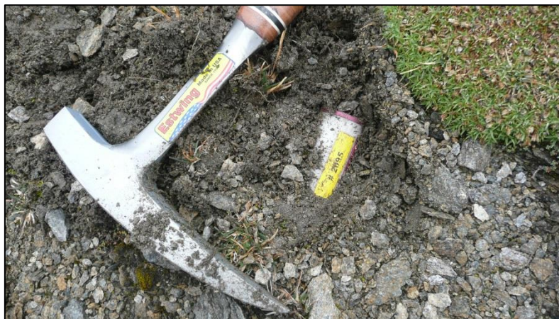
Figure 10: Miniature data logger for continuous GST measurements, placed in a depth of 10 cm to avoid direct radiation (Maurergrat, Kitzsteinhorn area).
