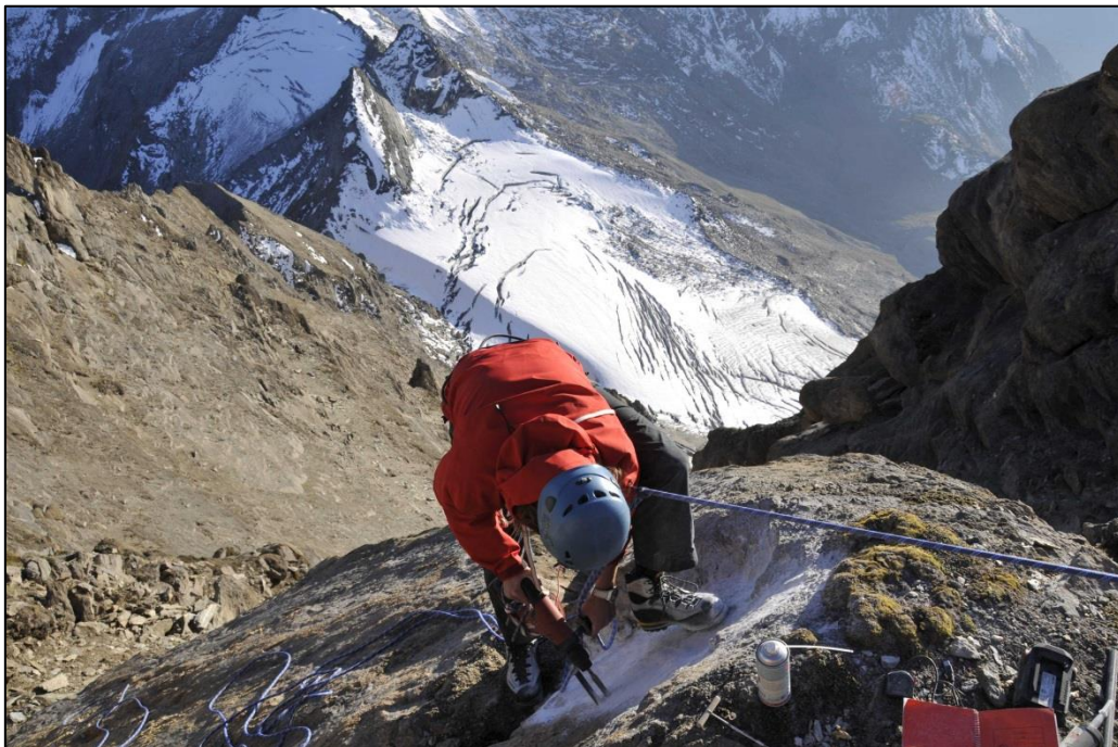
Figure 37: Drilling of a shallow borehole for iButton temperature measurement at the Kitzsteinhorn south face (Photograph by Ingo Hartmeyer).
