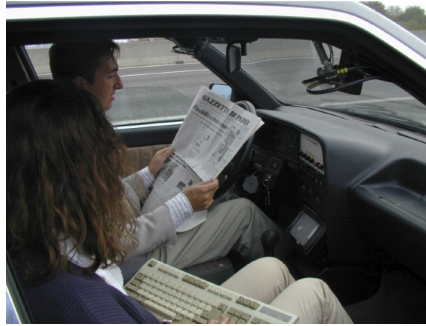
Fig. 1.5: ARGO Project, Universities of Parma and Pavia. An offshoot of the European PROMETHEUS project, the ARGO team drove their car about 2000 km around Italy in 1996, 94% of the time in autonomous mode. The special feature of this vehicle was the small number of sensors. With merely two black/white cameras the team achieved their goal. Image source: [173]
