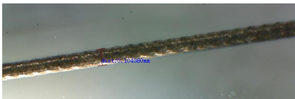
Figure 3.1: Line printed using a MOD silver ink on PET substrate. These continuous and smooth tracks are about 100 \mu\text{m} wide.
