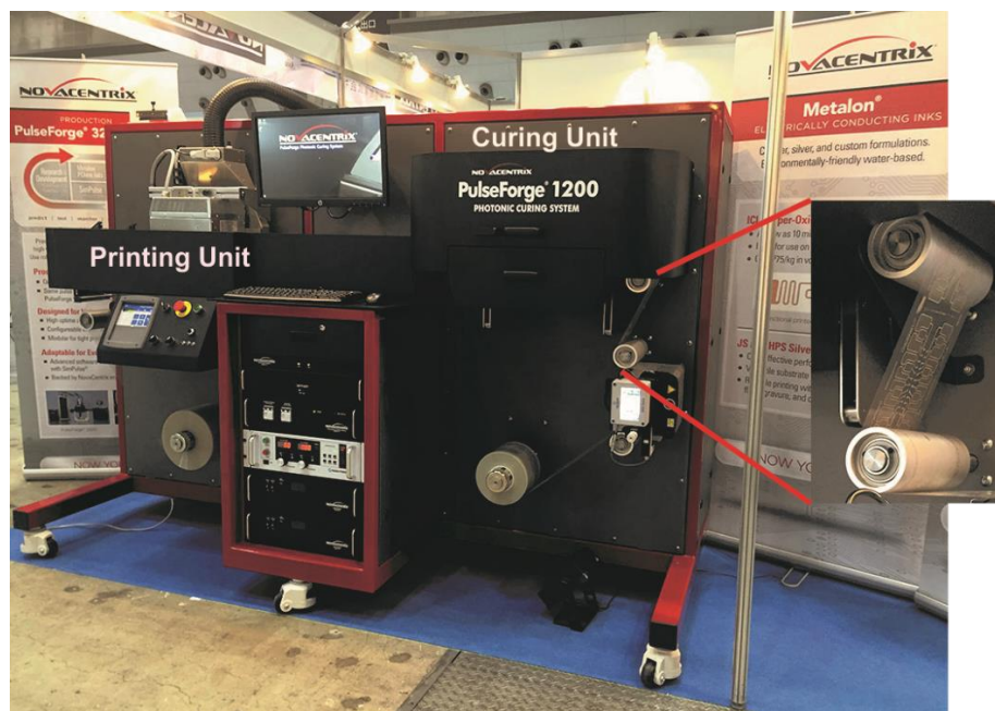
Figure 7.1: Pilot-scale roll-to-roll production line unit with an integrated printing, drying and photonic curing system from Novacentrix (Novacentrix, Austin).
