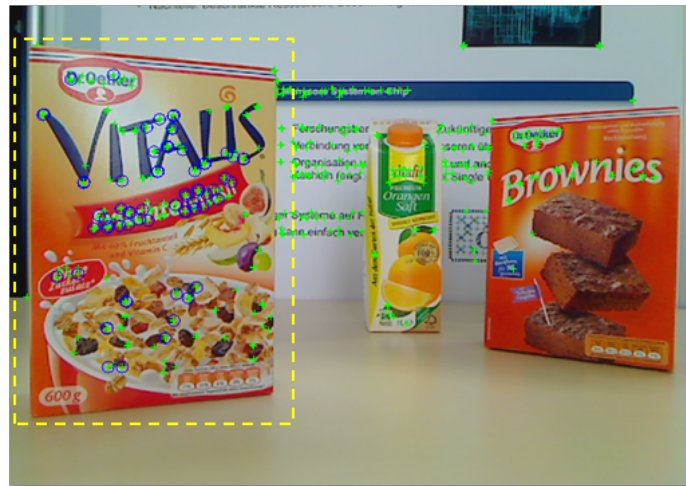
Figure 4.8.: Result from Harris-SIFT based object recognition technique
