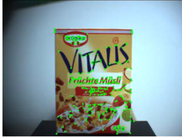
Figure 4.4.: Output from Harris Corner detection algorithm (detected corners are highlighted using green dots)
