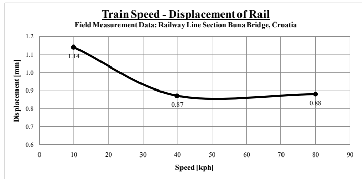
Figure 57: Example of running train test on a ballasted track in Zagreb, Croatia
