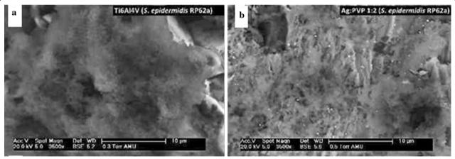
**Fig. 6** Biofilm formation on different Ti surfaces. Homogenous biofilm grade 5 after incubation with *S. epidermidis* on native Ti (**a**), reduced biofilm grade 3 on high concentrated Ag-DLC-Ti (**b**)
