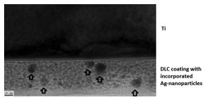
**Fig. 1** Transmission electron microscopy (TEM) image of silver nanoparticles of AG-DLC-Ti (note: major nanoparticles are marked with *arrows*)
