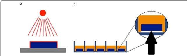
Fig. 2 Sample preparation; ion irradiation of samples with missing irradiation of the sample's lower surfaces (a), placement of samples in well culture plates with paraffin wax (arrow) covering the sample's lower surface (b)
