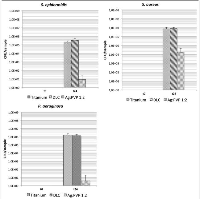
Fig. 3 Bacterial growth of tested strains on the sample surfaces (Ti, DLC-Ti, and high concentrated Ag-DLC-Ti); t = 0: before incubation; t = 24 h: after incubation
