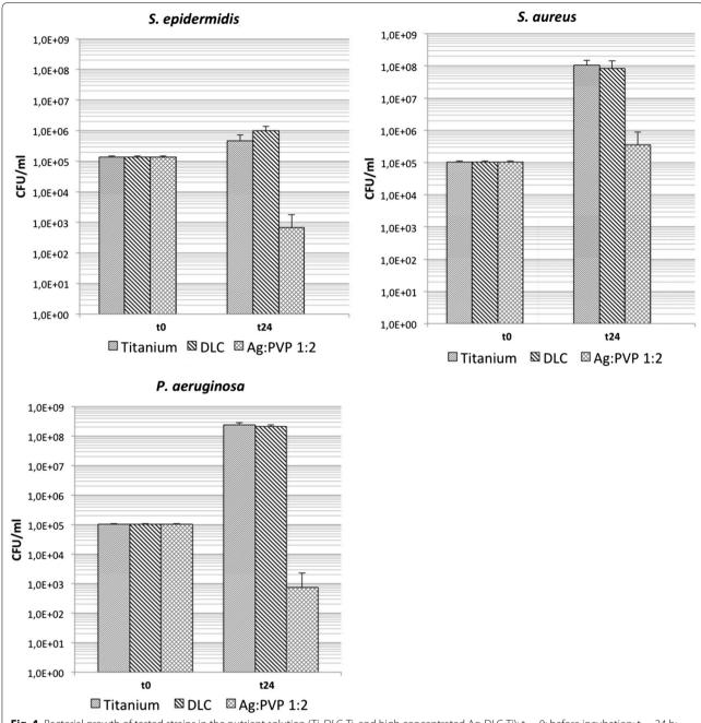
**Fig. 4** Bacterial growth of tested strains in the nutrient solution (Ti, DLC-Ti, and high concentrated Ag-DLC-Ti); t = 0: before incubation; t = 24 h: after incubation
